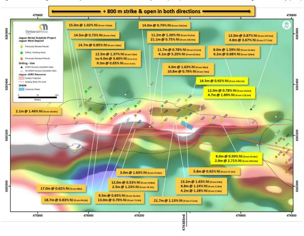
Figure 10 – The Jaguar West Deposit with DHEM conductor plates (blue) overlaid on the Ground Magnetics Survey (RTP)
