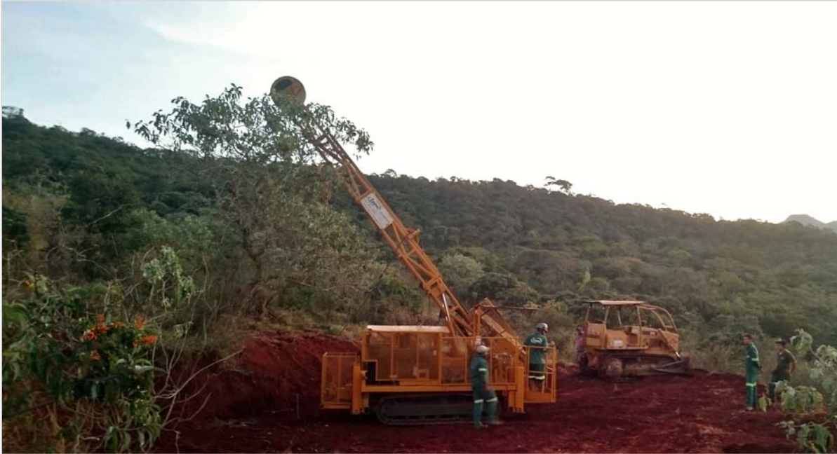
Figure 2 – Diamond drill rig on site at Mombuca Gold Project.
