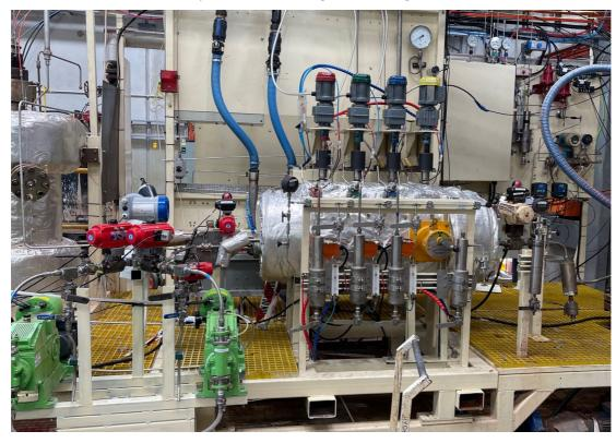
Figure 3: Pressure Leaching in Autoclave at ALS
