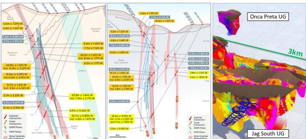
Figure 1. (A) Onca Preta and (B) Jag South sections showing deep drilling and (C) scoping UG design
