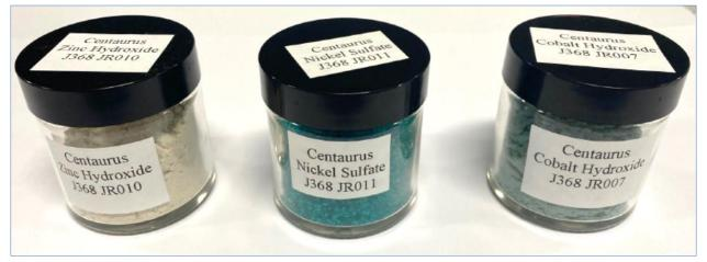
Figure 2. Zinc hydroxide, nickel sulfate and cobalt hydroxide from Jaguar refinery pilot testwork
