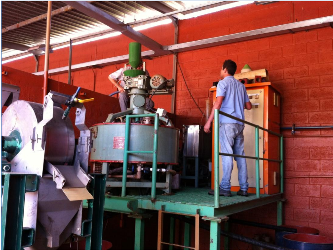
Figure 3 – Wet High Intensity Magnetic Separator (WHIMS) in Operation
