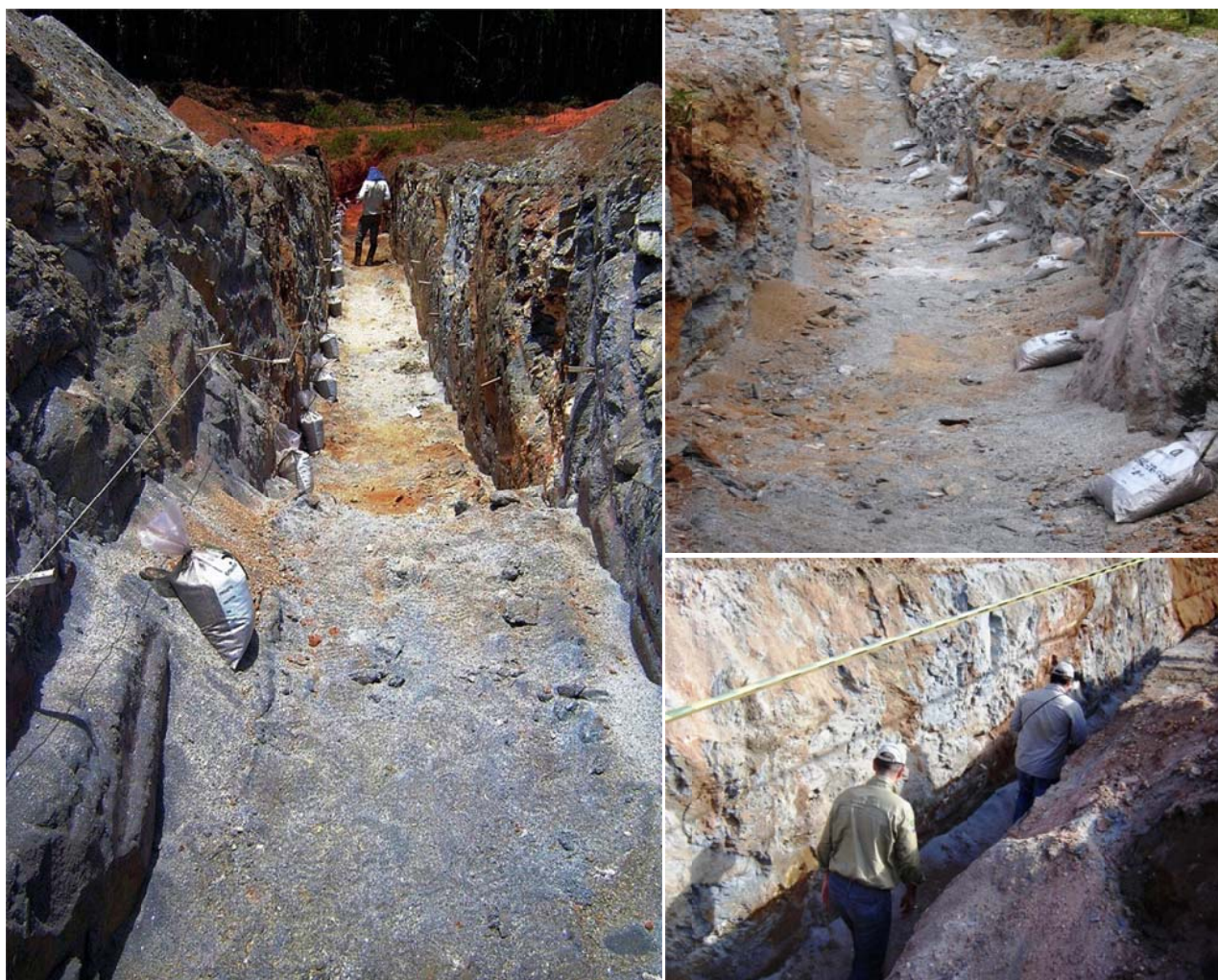
Figure 1 – Photos Showing Trenching across the Ore Zone at Tigre Prospect, Jambreiro.
