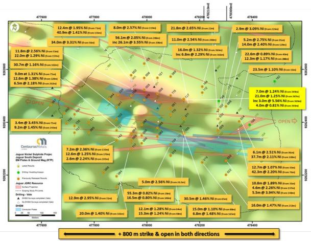
Figure 5 – The Jaguar South Deposit with DHEM conductor plates (blue) overlaid on the Ground Magnetics Survey (RTP)
