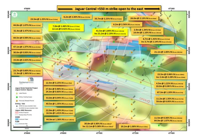
Figure 6 – The Jaguar Central Deposit with DHEM conductor plates (blue) overlaid on the Ground Magnetics Survey (RTP)
