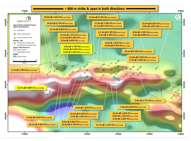
Figure 7 – The Jaguar West Deposit with DHEM conductor plates (blue) overlaid on the Ground Magnetics Survey (RTP)
