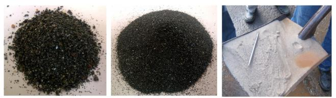
Figures 2, 3 & 4: (Left to Right) Jig Concentrate, WHIMS Cleaner Concentrate, Tails from WHIMS Cleaner Process
