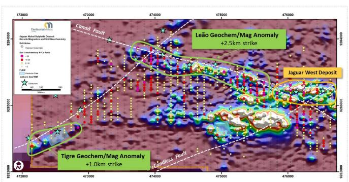
Figure 5 – The Leão & Tigre Prospects - Soils Geochemistry (Ni/Cr) and airborne GeoTEM Conductor picks (blue stars) over Ground Magnetics (Analytic Signal)
