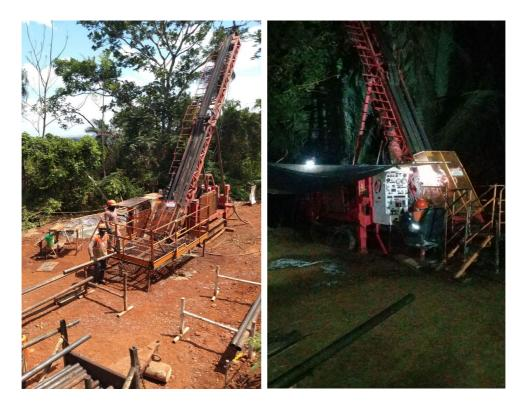
Figure 1 – Servdrill diamond rigs drilling day and night shift at the Jaguar Central and Onca Rosa Deposits.
