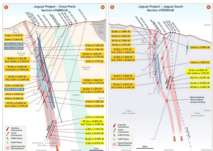
*Figure 13:* The Onça Preta Deposit: Cross-Sections 476885mE showing existing drilling, DHEM conductor plates in dark blue and FLEM conductor plates in light blue
