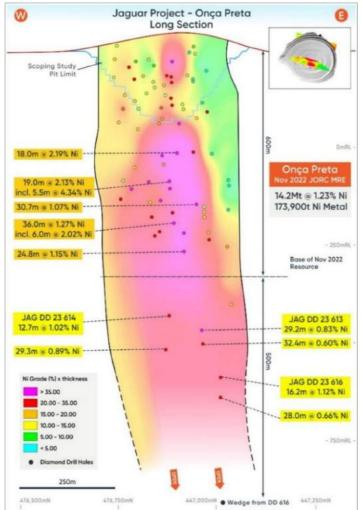
**Figure 12:** The Onça Preta Deposit long-section looking north showing location of recent Jaguar Deeps drill holes in relation to the base of the November 2022 MRE
