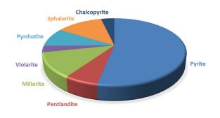
Figure 13: Average Sulphide Mineralogy of the Jaguar Nickel Project's Ore Zones
