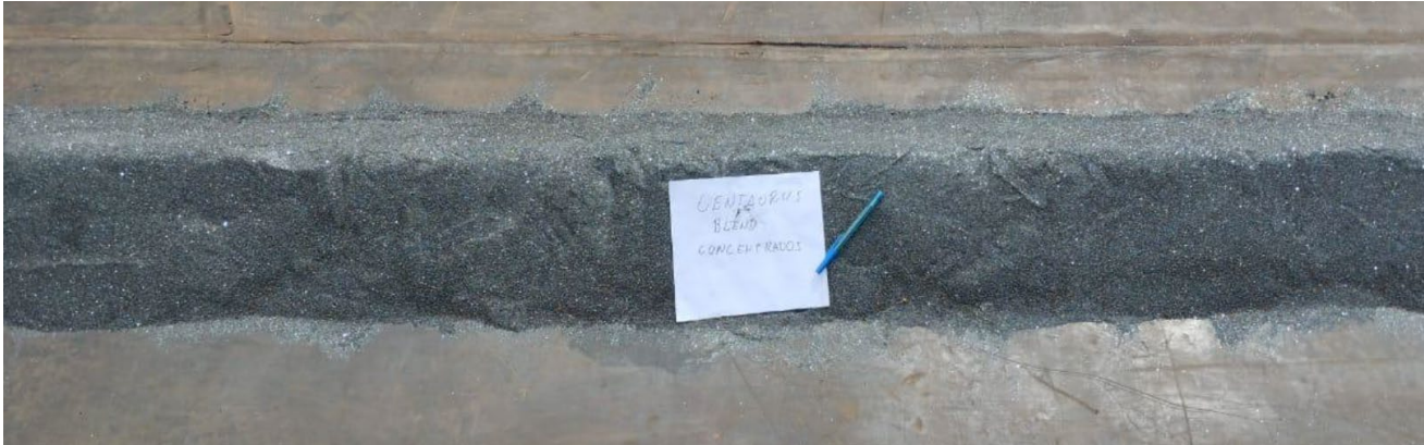
Figure 3 – Jambreiro DR-quality concentrate produced from pilot plant
