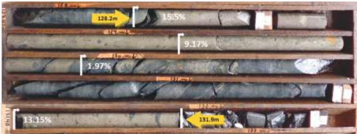
**Figure 3 - Core photos from drill hole JAG-DD-20-034; 128.2.2 to 131.9m: Semi-massive and massive sulphides** (metallic bronze/yellow) with magnetite (black) mineralisation hosted in altered dacite. Sulphides comprising pyrite, pentlandite, millerite, chalcopyrite and minor sphalerite. Interval returned 3.7m at 8.55% Ni, 0.43% Cu and 0.12% Co from 128.2m
