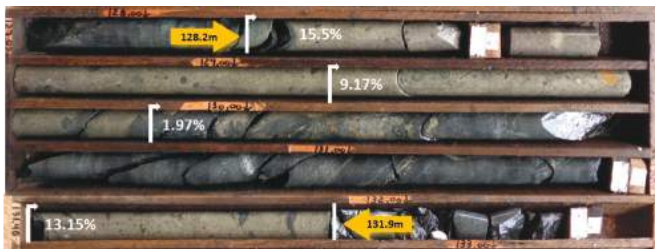
Figure 3 - Core photos from drill hole JAG-DD-20-034; 128.2.2 to 131.9m: Semi-massive and massive sulphides
