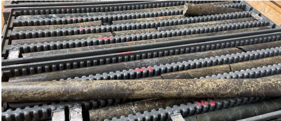
Figure 7 – Core from drill hole JAG-DD-21-190 (Onça Preta): Semi-massive and massive sulphides (metallic bronze/yellow colour), predominantly pyrite, millerite and pentlandite, with intense magnetite alteration hosted in the basement granite.
