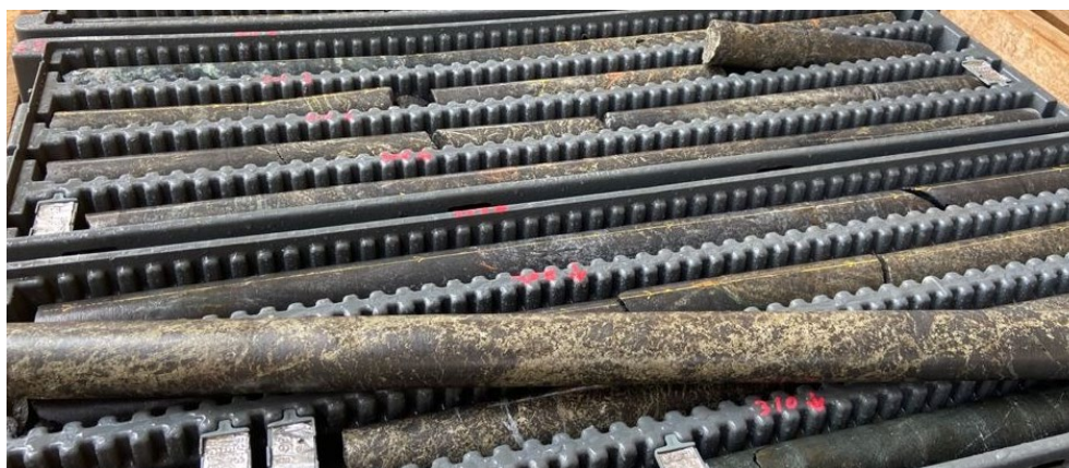
Figure 1 – Core from drill hole JAG-DD-21-190 (Onça Preta): Semi-massive and massive sulphides (metallic bronze/yellow colour), predominantly pyrite, millerite and pentlandite, with intense magnetite alteration hosted in the basement granite.
