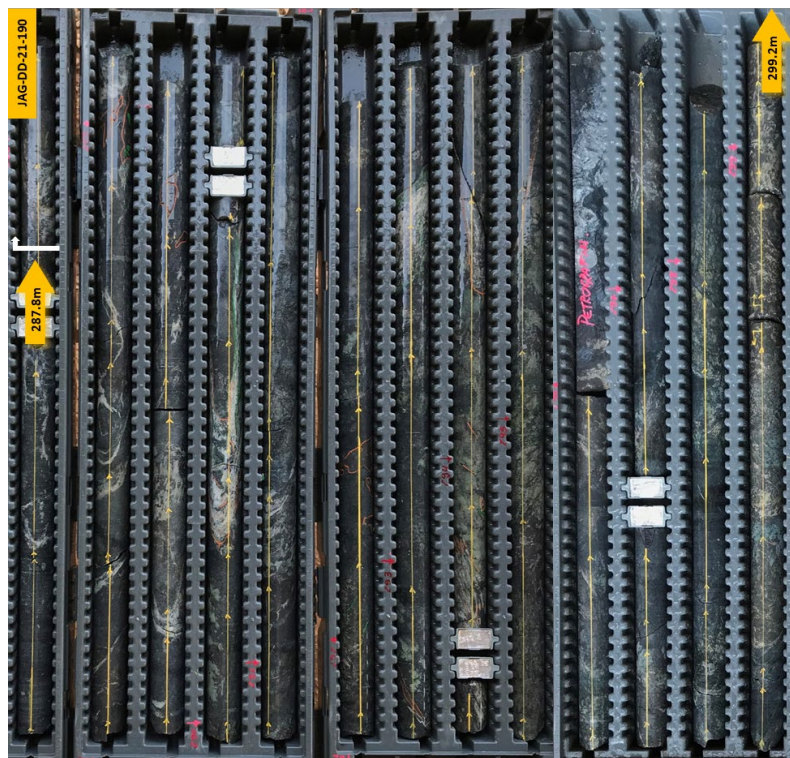
Figure 7 – Core photo from drill hole JAG-DD-21-190 (Onça Preta); 287.8m to 309.9m down-hole: Disseminated, stringer to semi-massive sulphides (metallic bronze/yellow colour) with intense magnetite (black colour) mineralisation hosted in basement gneiss.
